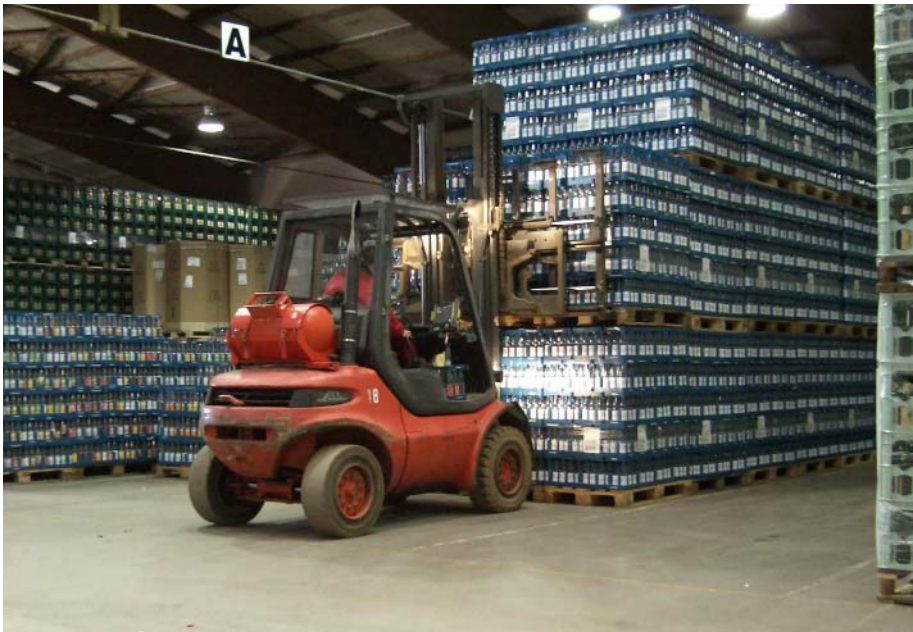
In average, four fork lifters - two double and two triple lifters - are in use for putaway, retrieval and replenishment.
