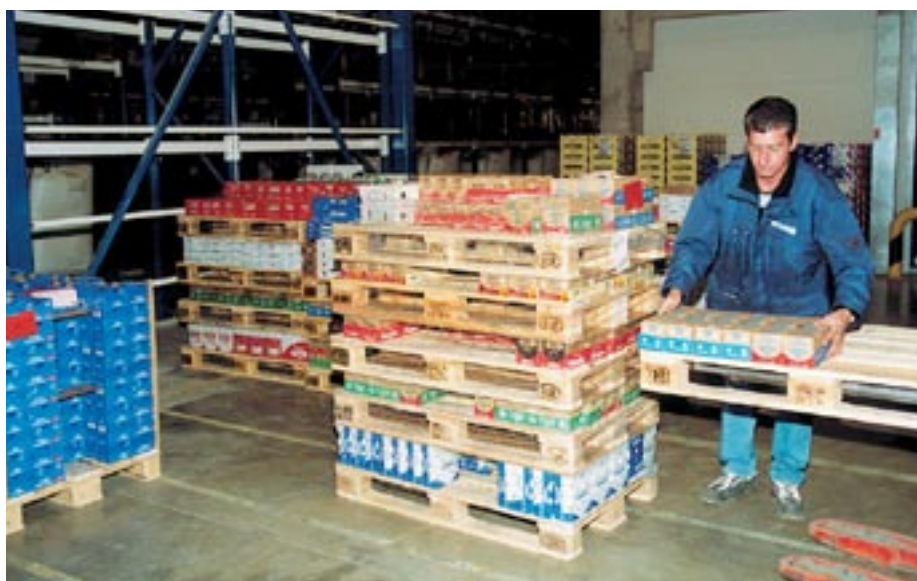
For clients that have arranged a certain pallet height for delivery, the full pallets' height is reduced down to the desired height by employees before release
