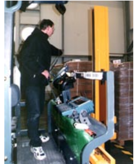
Scanning of goods in the high-bay warehouse
